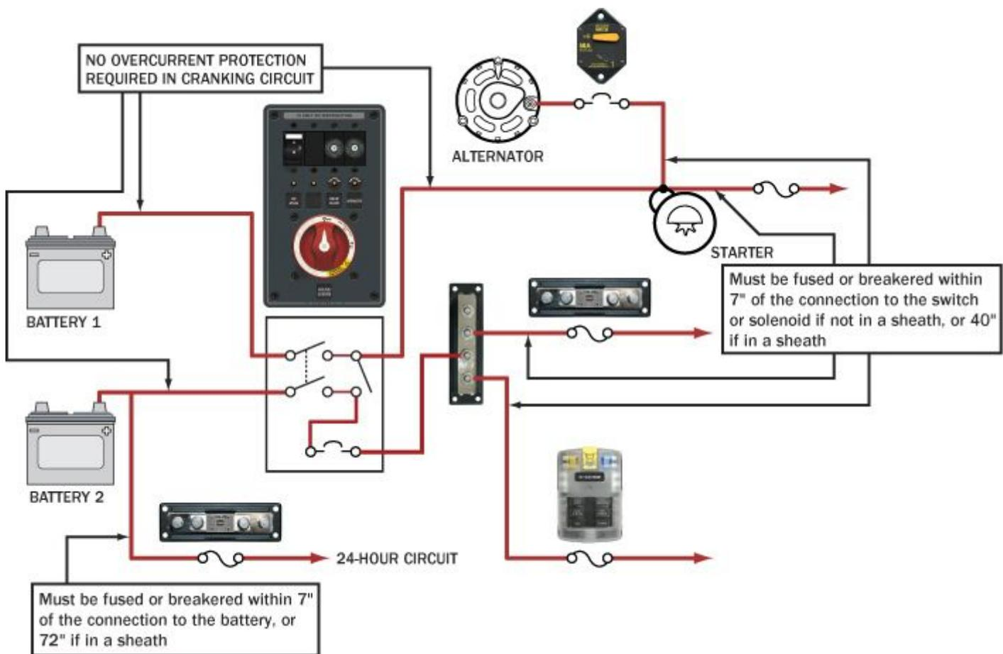
Notice that wires intended to carry engine-starting currents between the batteries, the switch, and the starter, are not required to have main-circuit-protection devices installed.
