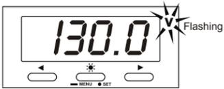
The present setting will appear in the display (Default 130.0). If the set point is acceptable, press the \* button or wait for 15 seconds and the meter will revert to normal operation. Otherwise use the ◀ arrow ▶ buttons to select the desired value. For example, press and hold the right ▶ button to scroll up to 250 Volts.
