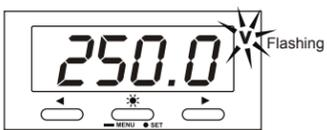
Press the \* button when the desired set point is displayed and the new value will be saved to memory. Two short beeps will let you know you have successfully set the new value and the meter will revert to normal operation.
